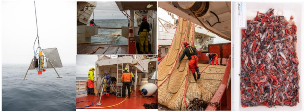
Figure 3.2.3: Images of some of the instruments used to sample backscatter and macrozooplankton and nekton for the MEESO project. WBT-TUBE submersible echosounder (left image and lower middle image), pelagic trawl being deployed (upper middle image) and retrieving trawl and main catch (right images). Photos by Svanhildur Egilsdóttir.
