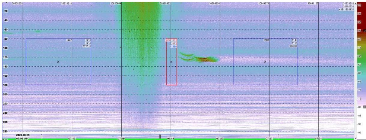
Fig. 3.1.2. Echogram from acoustic mooring showing the passing of the vessel (noise band starting at 07:15) and the trawl (strong echo in midwater around 07:20), and periods before and after. Boxes in midwater depths show locations of integration bins used in analysis.
