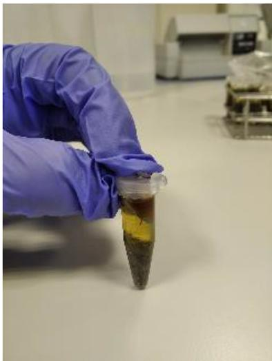
*Figure 6 Phase separation after centrifugation of a sample.*
