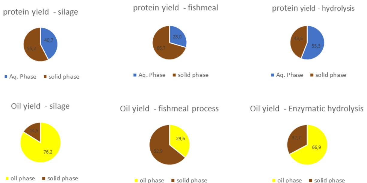
Figure 8 Oil and protein recovery as a result of process. Yields are percentages of the amounts of protein and lipids in the raw material and do not sum to 100% because of losses in the processing
