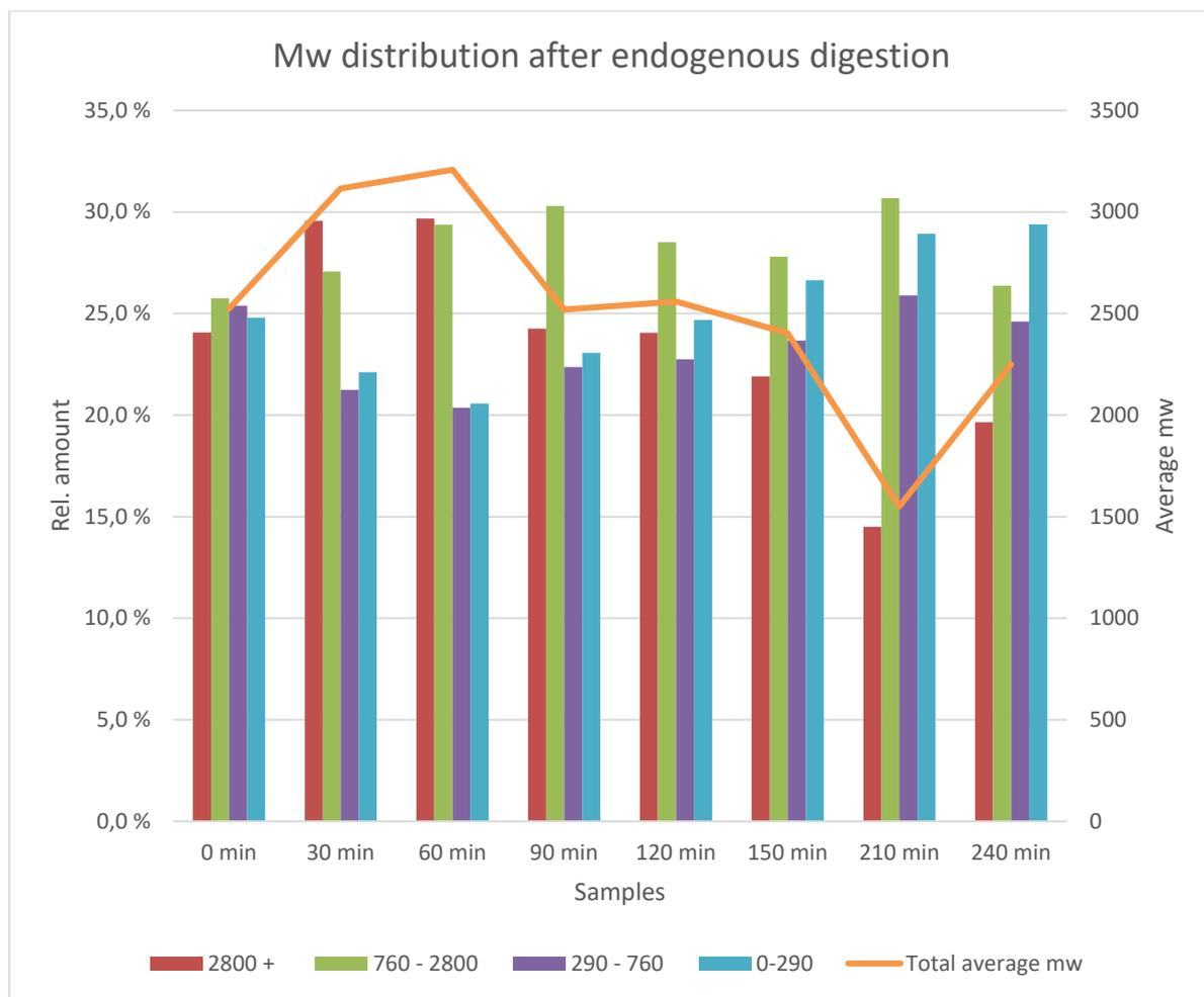
Figure 10 mw distribution of hydrolysate of Mp after four h hydrolysis. samples taken every 30 min. The green trace is average mw.
