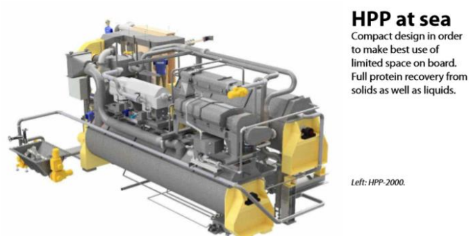
Figure 10: Example of onboard system to process fish oil and fish meal. Source: Hedinn.
